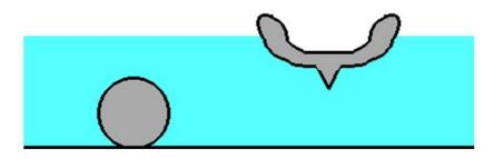
Displaced water less than ball weight
