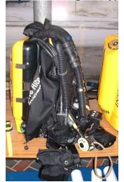
That's called a "rebreather" or "closed-circuit" oxygen system. In layman's terms...a rebreather is an oxygen tank that absorbs the carbon dioxide that we exhale when we breathe and recycles it by mixing it with pure oxygen so it can be reused by the user. This differs from an open-circuit breathing apparatus, where the exhaled carbon dioxide is discharged directly into the environment. Oh those climbers were only 329 feet away.
