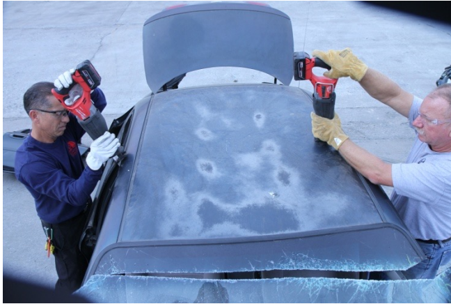
RELIEF CUT ON ROOF IN FRONT OF "B" POST
