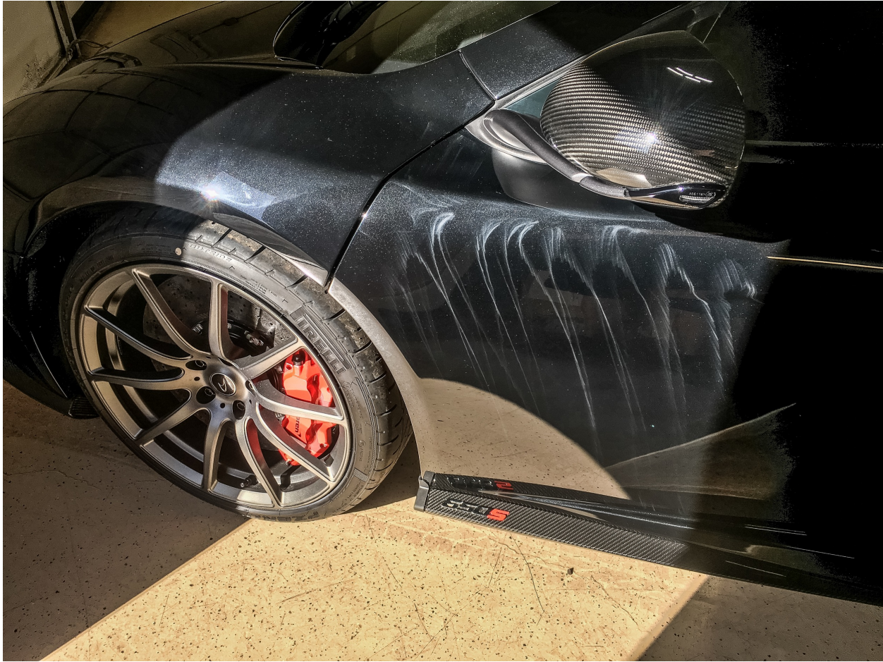
A buffer used incorrectly
