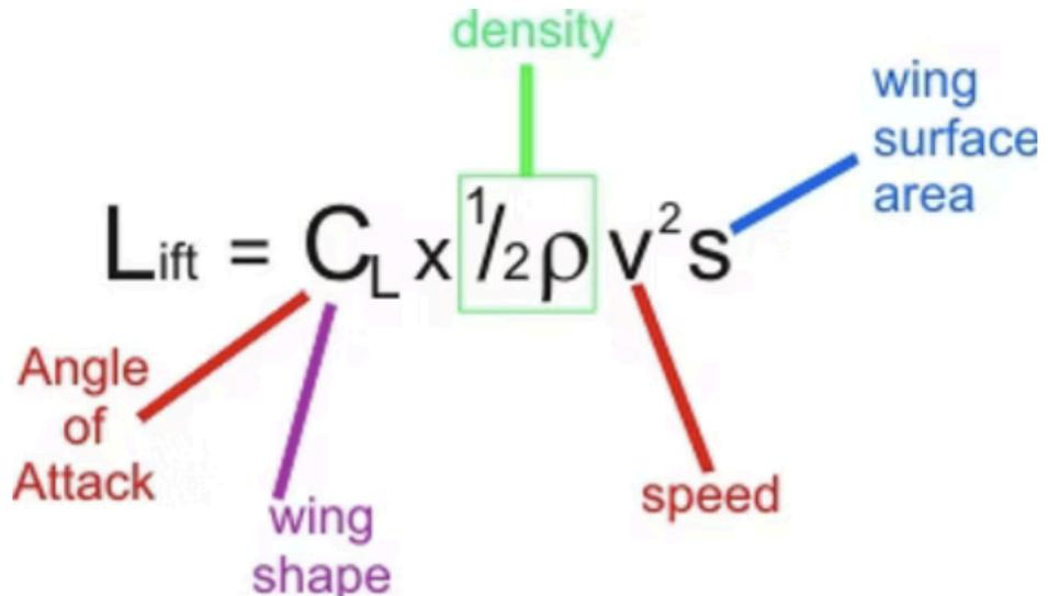
The diagram illustrates the lift equation with five variables: density (green), wing surface area (blue), speed (red), wing shape (purple), and angle of attack (red). The variables are arranged around the equation, with lines pointing from the labels to the corresponding terms in the equation.
