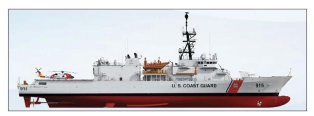
This is our new Offshore Patrol Cutter, a few of which are being constructed now. Each of these will be 360 feet long and displace between 3,700 and 4,500 tons. The white section is what you would see above the water while the red area at the bottom is the part that would be under the water.
